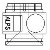
1 Body 35mmx33mm With Flat Bottom for Universal Mounting Plate
